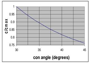
**Fig.3.** The ratio  $c/c_{\text{max}}$  vs. con angle.
